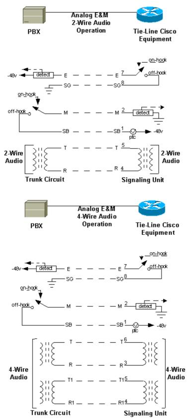
**Note:** For the four–wire audio setup, Pin 6 (Tip) and 3 (Ring) on the router transport the audio path from the PBX to the router. Pin 5 (Tip1) and 4 (Ring1) on the router transport the audio path from the router to the
