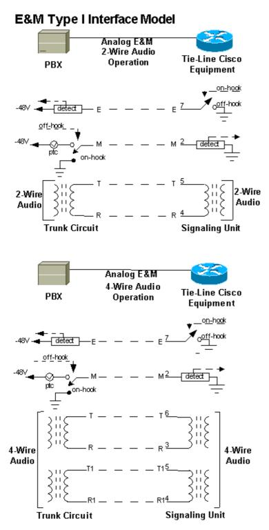
**Note:** For the four–wire audio setup, Pin 6 (Tip) and 3 (Ring) on the router transport the audio path from the PBX to the router. Pin 5 (Tip1) and 4 (Ring 1) on the router transport the audio path from the router to the PBX.
