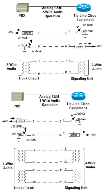
**Note:** For the four–wire audio setup, Pin 6 (Tip) and 3 (Ring) on the router transport the audio path from the PBX to the router. Pin 5 (Tip1) and 4 (Ring1) on the router transport the audio path from the router to the PBX.
