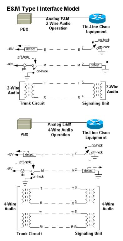
**Note:** For the four–wire audio setup, Pin 6 (Tip) and 3 (Ring) on the router transport the audio path from the PBX to the router. Pin 5 (Tip1) and 4 (Ring 1) on the router transport the audio path from the router to the PBX.
