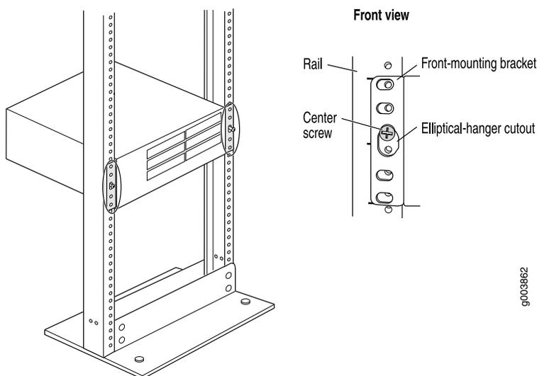
4. Install at least two mounting screws into each mounting bracket, in addition to the center screws from which the router hangs.
