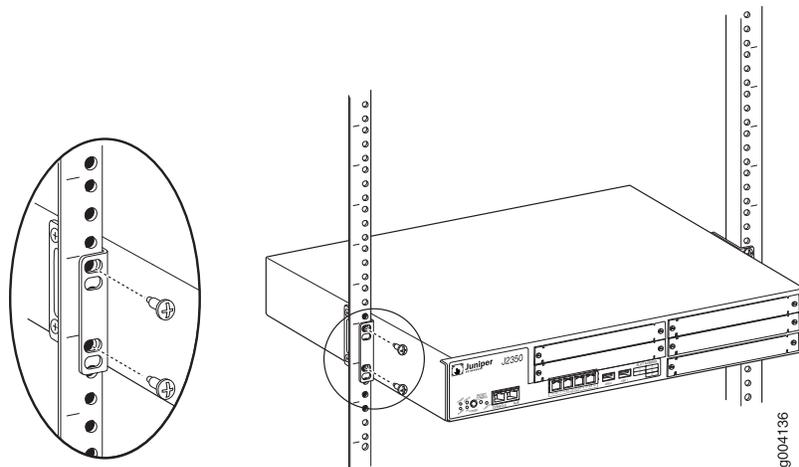
3. Have a second person install a mounting screw into each of the two aligned holes. With a number 2 Phillips screwdriver, tighten the screws.
