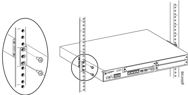
**Figure 4: Hanging a J2350 Router in a Rack**
