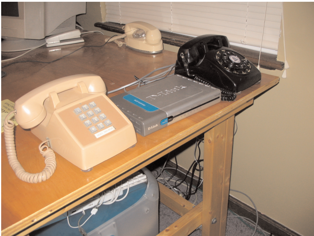
Figure 2.3 A D-Link Analog Telephone Adapter Controlling Two Older Analog Phones
