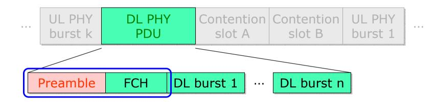
The DL subframe starts with a preamble (necessary for frame synchronization and equalization) and the Frame Control Header (FCH) that contains the location and burst profile of the first DL burst following the FCH. The FCH is one OFDM symbol long and is transmitted using BPSK modulation.
