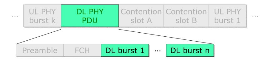
A subscriber station (SS) does not know which DL burst(s) contain(s) information sended to it, since the Connection ID (CID) is located in the MAC header, not in the DL PHY PDU header.
