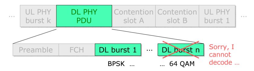
A subscriber station (SS) listens to all bursts it is capable of receiving (this includes bursts with profiles of equal or greater robustness than has been negotiated with the base station at connection setup time).
