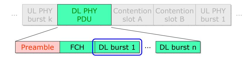
The first burst in downlink contains the downlink and uplink maps (DL MAP & UL MAP) and downlink and uplink channel descriptors (DCD & UCD). These are all contained in the first MAC PDU of this burst. The burst may contain additional MAC PDUs.
