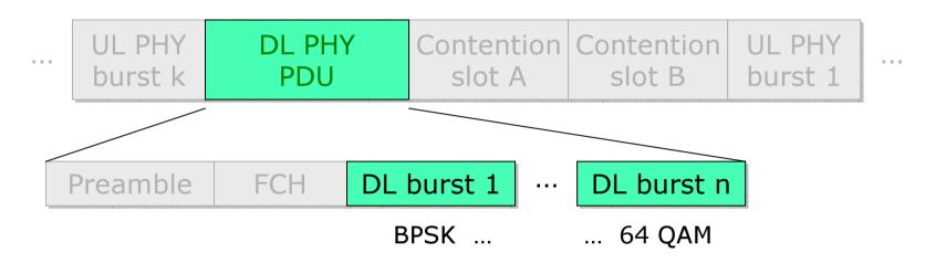
Downlink bursts are transmitted in order of decreasing robustness. For example, with the use of a single FEC type with fixed parameters, data begins with BPSK modulation, followed by QPSK, 16-QAM, and 64-QAM.
