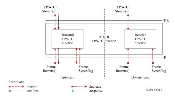
Figure 6-2/G.992.3 – Signals of an ATU-R TPS-TC function
