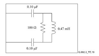
NOTE - Component Tolerances: Capacitors: 2.5%, Resistors: 1%, Coils: 5%.
