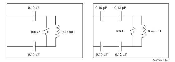
NOTE - Component tolerances: Capacitors: 2.5%, Resistors: 1%, Coils: 5%.
