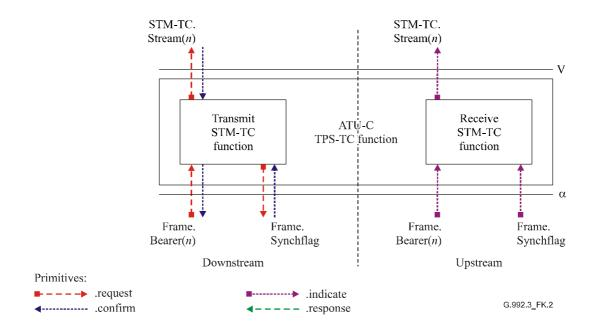
Figure K.2/G.992.3 – Signals of the ATU-C STM-TC function
