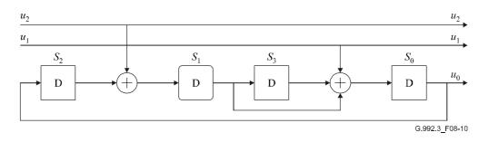
Figure 8-10/G.992.3 – Finite state machine for Wei's encoder
