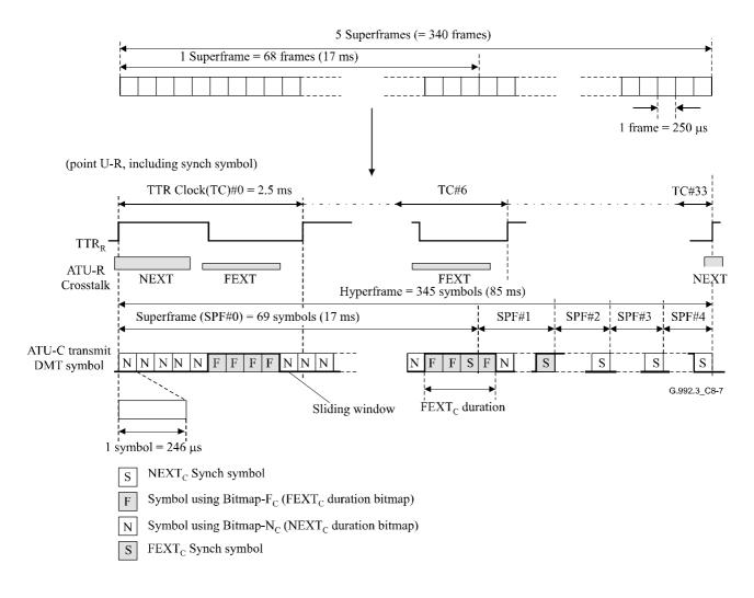
Figure C.8-7/G.992.3 – Hyperframe structure for upstream
