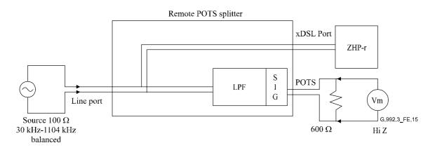
Figure E.15/G.992.3 – Measurement of the remote splitter attenuation in the ADSL band
