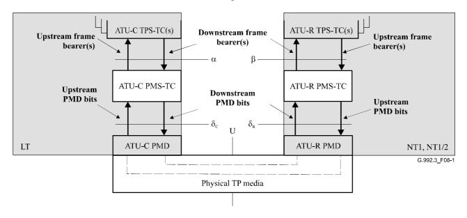
Figure 8-1/G.992.3 – PMD transport capabilities within the data plane
