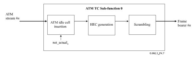
Figure K.7/G.992.3 – Block diagram of transmit ATM-TC function
