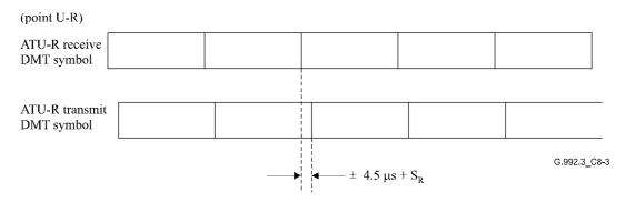
Figure C.8-3/G.992.3 – Loop timing for ATU-R
