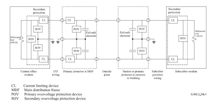
Figure III.1/G.992.3 – Typical arrangement of protection devices
