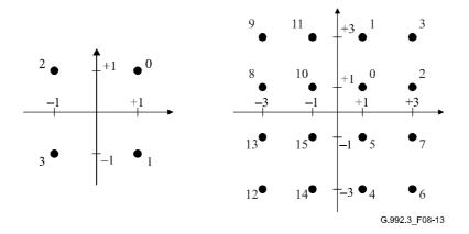
Figure 8-13/G.992.3 – Constellation labels for b = 2 and b = 4
