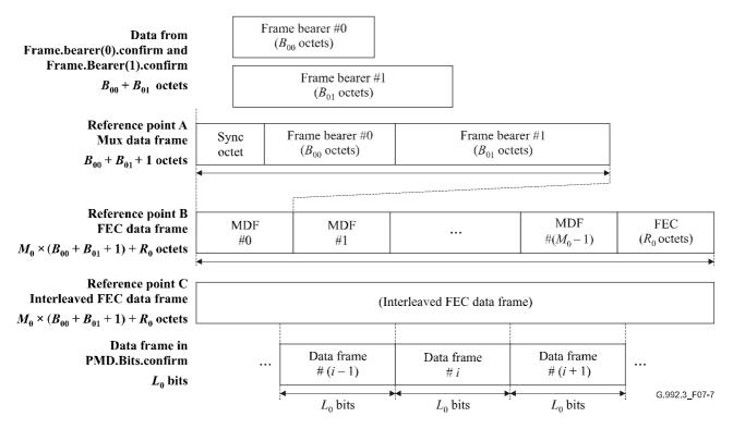
Figure 7-7/G.992.3 – Illustration of frame structure with single latency dual bearers and  $T_p = 1$
