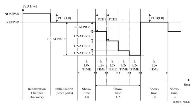
Figure 9-4a/G.992.3 – Illustration of the L2 power state control parameters
