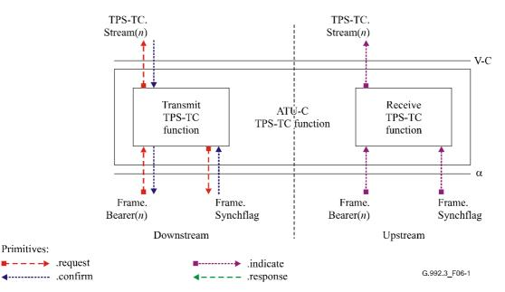
Figure 6-1/G.992.3 – Signals of an ATU-C TPS-TC function
