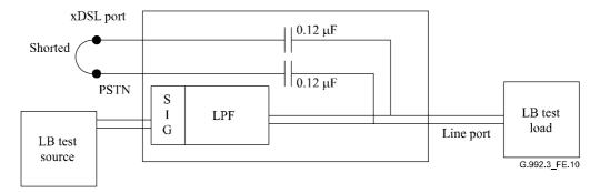
Figure E.10/G.992.3 – Longitudinal balance CO test setup
