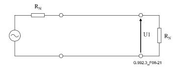
Figure 8-21/G.992.3 – Voltage across the load
