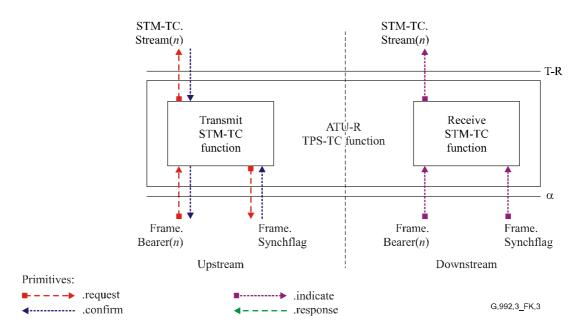
Figure K.3/G.992.3 – Signals of the ATU-R STM-TC function
