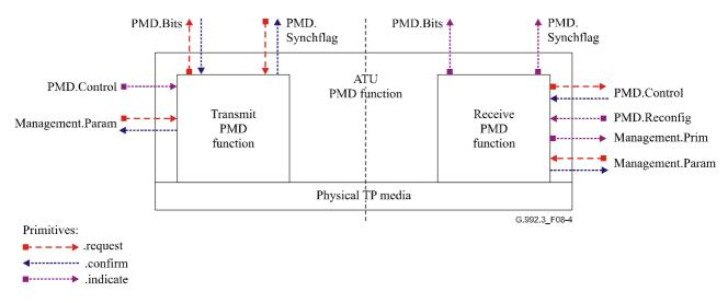
Figure 8-4/G.992.3 – Signals of the ATU PMD function
