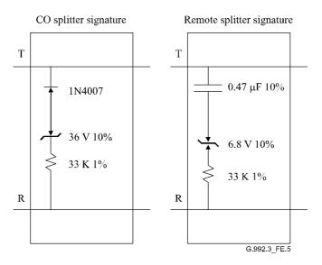
Figure E.5/G.992.3 – Maintenance test signatures
