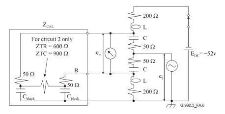
Figure A.6/G.992.3 – Calibration circuit
