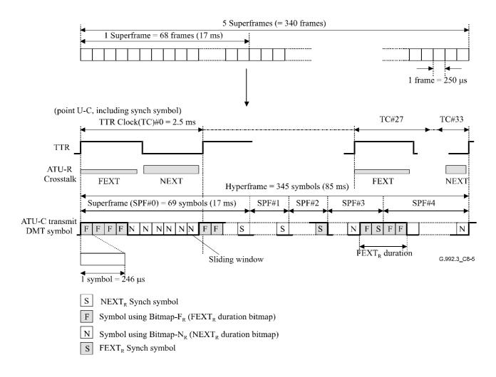
Figure C.8-5/G.992.3 – Hyperframe structure for downstream
