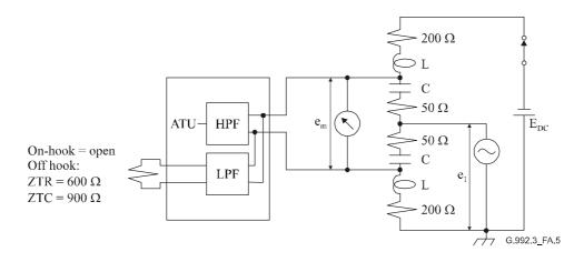
Figure A.5/G.992.3 – Longitudinal balance above 30 kHz measurement method (HPF and LPF integrated)
