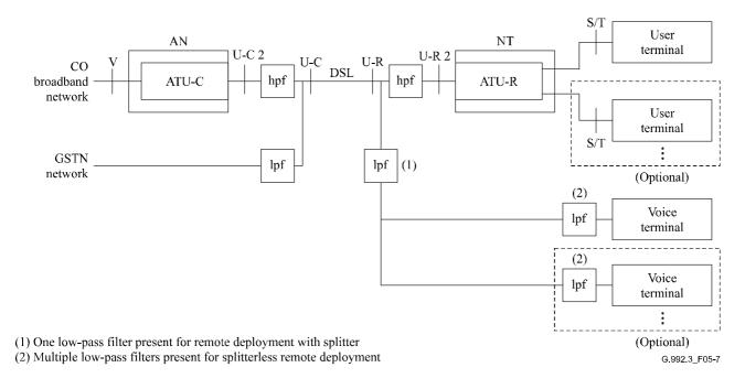
Figure 5-7/G.992.3 – Data with POTS service application model
