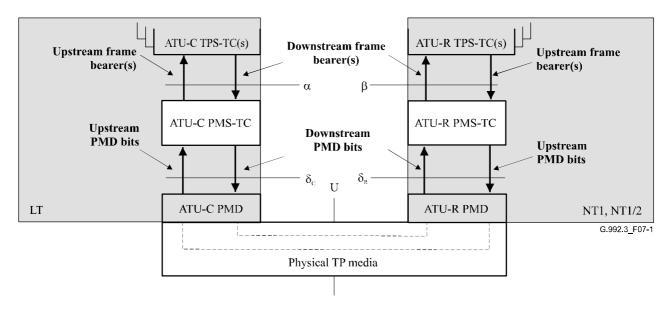
Figure 7-1/G.992.3 – PMS-TC transport capabilities within the user plane
