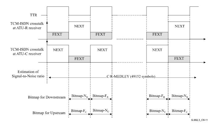
Figure C.8-11/G.992.3 – Estimation of periodic signal-to-noise ratio
