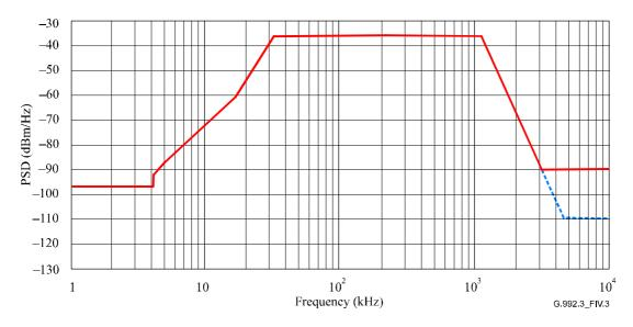
Figure IV.3/G.992.3 – A shaped downstream PSD mask for profile 3
