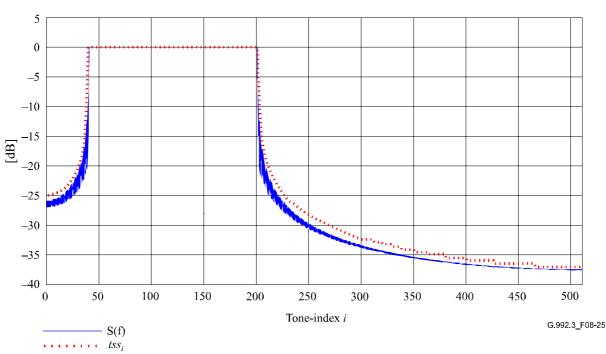
Transmit spectrum shaping values and downstream spectrum S(f) [40, 200]
