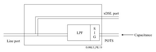
Figure E.13/G.992.3 – Capacitance test
