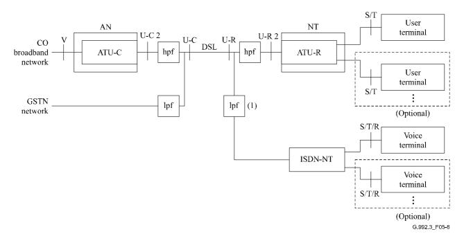
Figure 5-8/G.992.3 – Data with ISDN service application model
