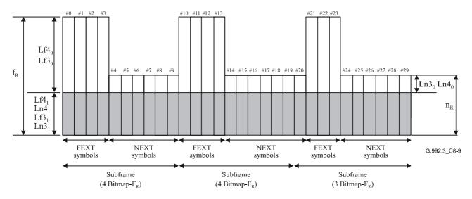
Figure C.8-9/G.992.3 – First example of data rate to symbol type mapping
