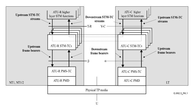
Figure K.1/G.992.3 – STM-TC transport capabilities within the user plane
