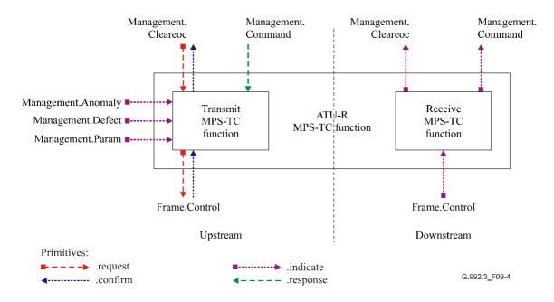
Figure 9-4/G.992.3 – Signals of the ATU-R MPS-TC function
