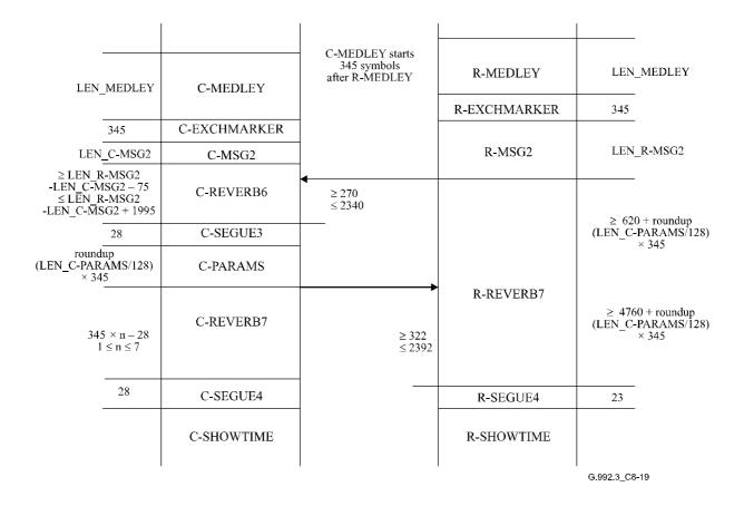
Figure C.8-19/G.992.3 – Timing diagram of the initialization procedure (part 2) with C-PARAMS and without R-PARAMS states
