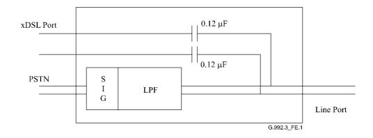
Figure E.1/G.992.3 – External POTS central office splitter without HPF function
