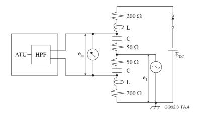
Figure A.4/G.992.3 – Longitudinal balance above 30 kHz measurement method (only HPF integrated)
