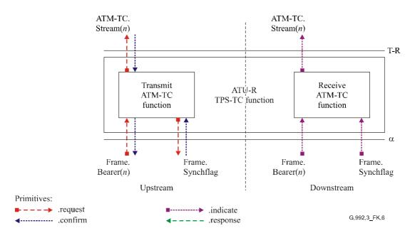
Figure K.6/G.992.3 – Signals of the ATU-R ATM-TC function
