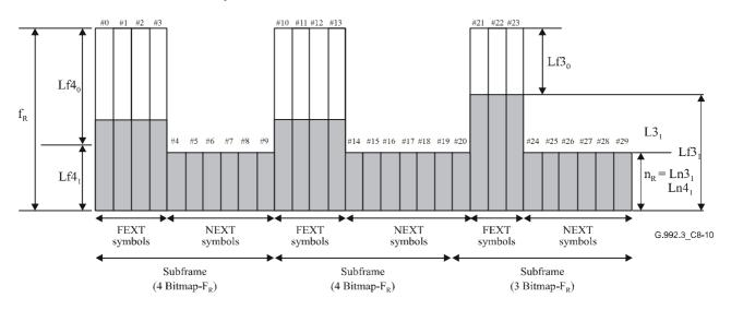
Figure C.8-10/G.992.3 – Second example of data rate to symbol type mapping
