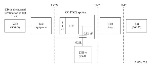
ZHP-c = the impedance presented to the POTS connection by an ATU-C through the capacitance of the POTS splitter DC blocking capacitors
