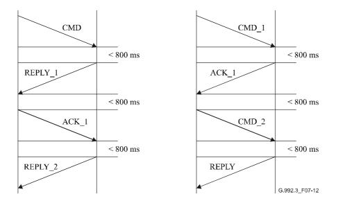
Figure 7-12/G.992.3 – Example of segmentation of a command and response of priority 2 in two segments
