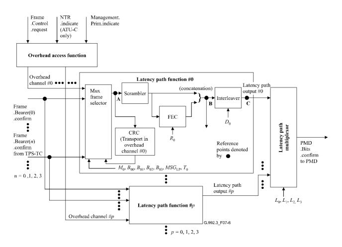
Figure 7-6/G.992.3 – Block diagram of transmit PMS-TC function
