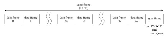
Figure 8-6/G.992.3 – ADSL superframe structure – ATU-C transmitter
