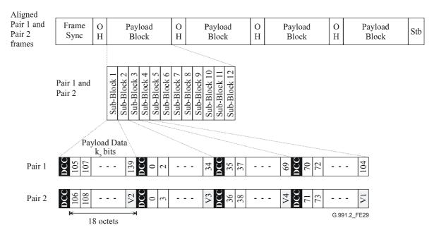
Figure E.29/G.991.2 – *M*-Pair TU-12 framing with a data communication channel (N = 1 TU-12 links with i = 1 over M = 2 wire-pairs)
