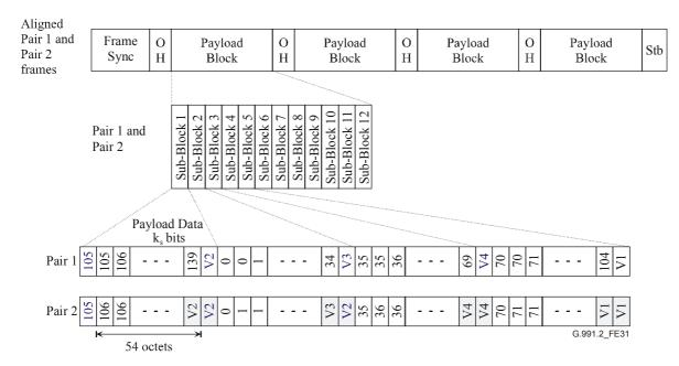
Figure E.31/G.991.2 – *M*-Pair TU-12 Framing with a data communication channel (*N* = 3 TU-12 links with *i* = 0 over *M* = 2 wire-pairs)
