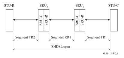
Figure D.1/G.991.2 – Block diagram of a SHDSL span with two signal regenerators
