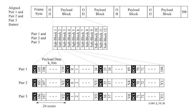
Figure E.30/G.991.2 – *M*-Pair TU-12 framing with a data communication channel (N = 2 TU-12 links with i = 1 over M = 3 wire-pairs)
