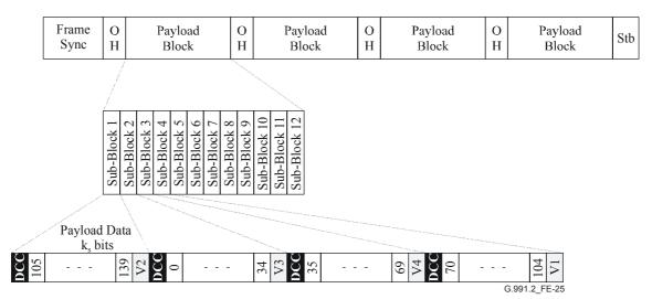
NOTE – V1, V2 and V3 are TU-12 pointers 1, 2 and 3; V4 is set to ONE. These bytes are part of the TU-12 and terminated at a pointer processor.
