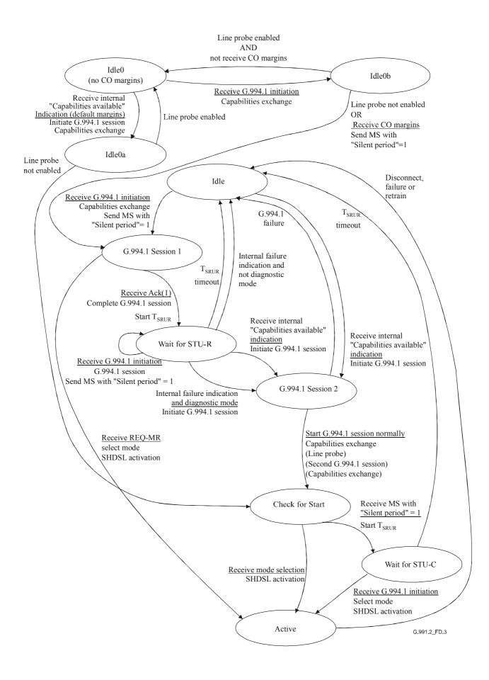
Figure D.3/G.991.2 – SRU-R state transition diagram
