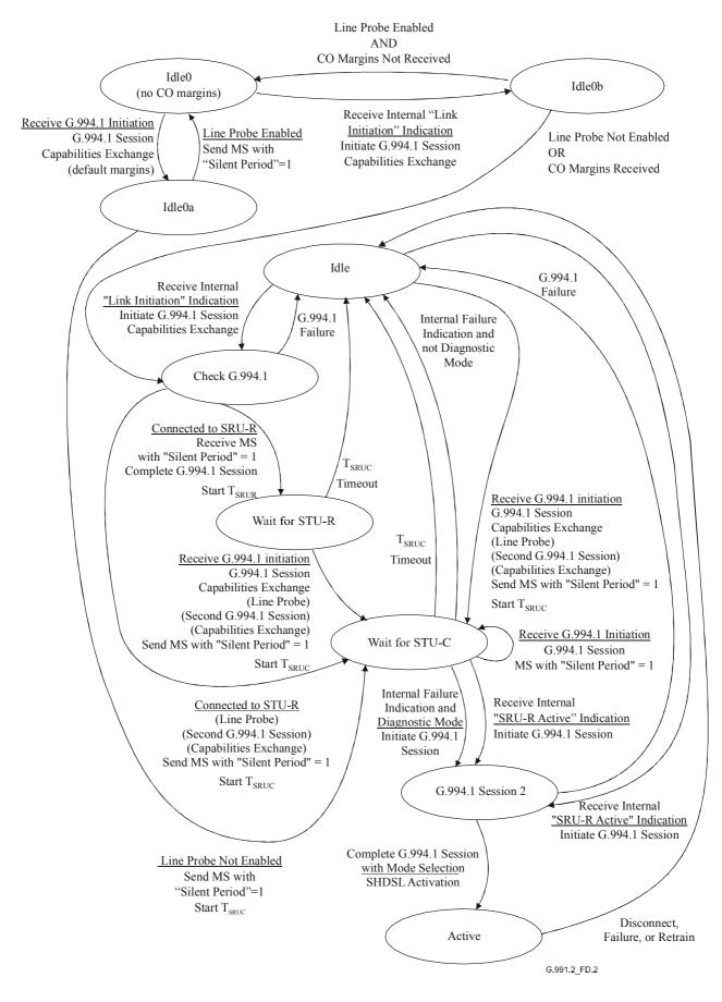
Figure D.2/G.991.2 – SRU-C state transition diagram
