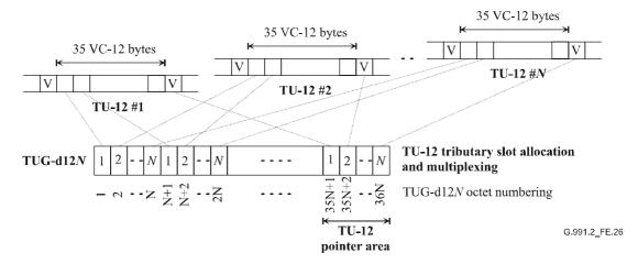
Figure E.26/G.991.2 – Arrangement of  $N \times$  TU-12s multiplexed into a TUG-d12N (N = 1, 2, ..., 9)
