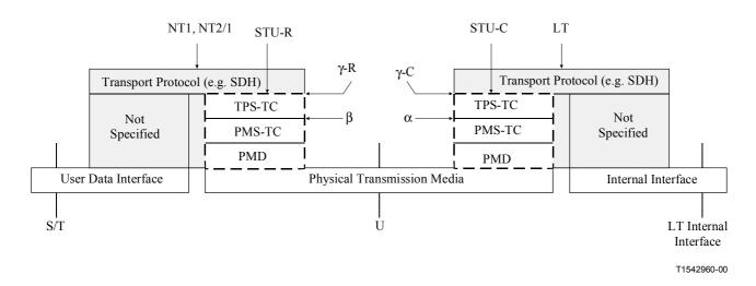
Figure 12/G.995.1 – User plane protocol reference architecture for ITU-T G.991.2
