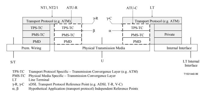
Figure 9/G.995.1 – User plane protocol reference architecture
