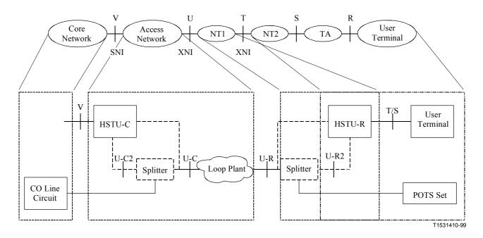
Figure 6/G.995.1 – G.994.1 system reference model and its alignment with the generic reference configuration
