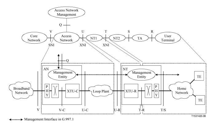
Figure 7/G.995.1 – G.997.1 system reference model and its alignment with the generic reference configuration
