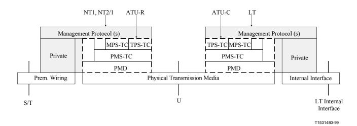
Figure 14/G.995.1 – Management plane protocol reference architecture for G.99x Recommendations
