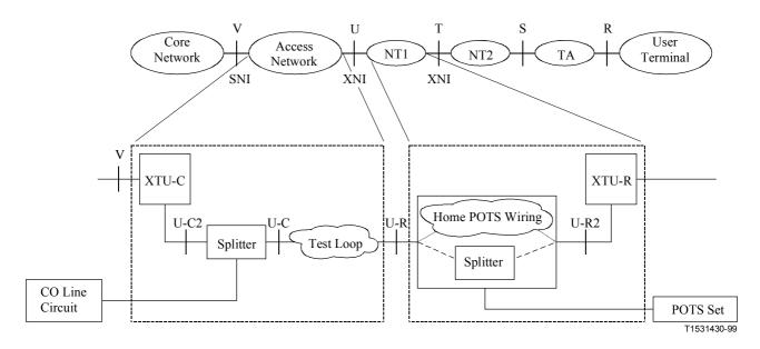
Figure 8/G.995.1 – G.996.1 system reference model and its alignment with the generic reference configuration
