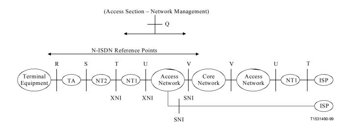
Figure 15/G.995.1 – Illustration of a generic xDSL data Connection
