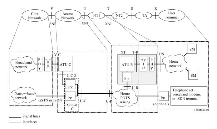
Figure 3/G.995.1 – G.992.2 system reference model and its alignment with the generic reference configuration
