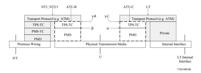
Figure 10/G.995.1 – User plane protocol reference architecture for ITU-T G.992.1 and G.992.2
