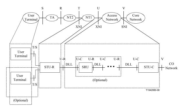
Figure 5/G.995.1 – G.991.2 system reference model and its alignment with the generic reference configuration
